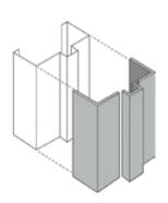
Note: Sheet thickness should be taken into account in calculation of sizes. We will require internal dimensions of the frame protection required.
